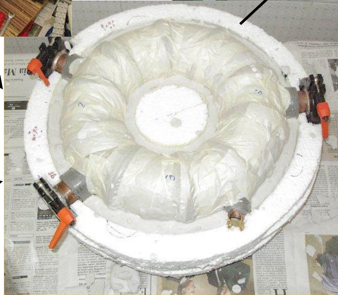
Vacuum vessel wrapped (thermal expansion layer) inside the mould. Plaster is poured.
