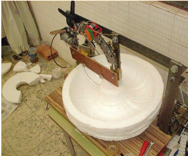
Creating the porexpan mould
