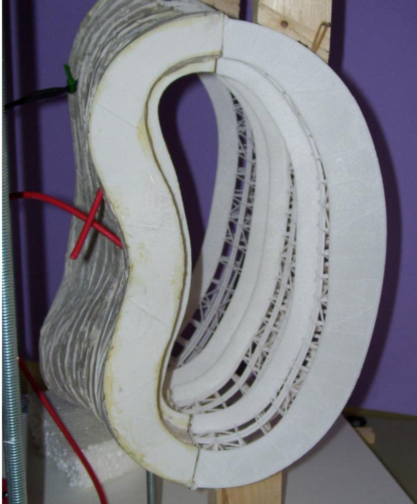
Two views of the test of a coil frame sector
